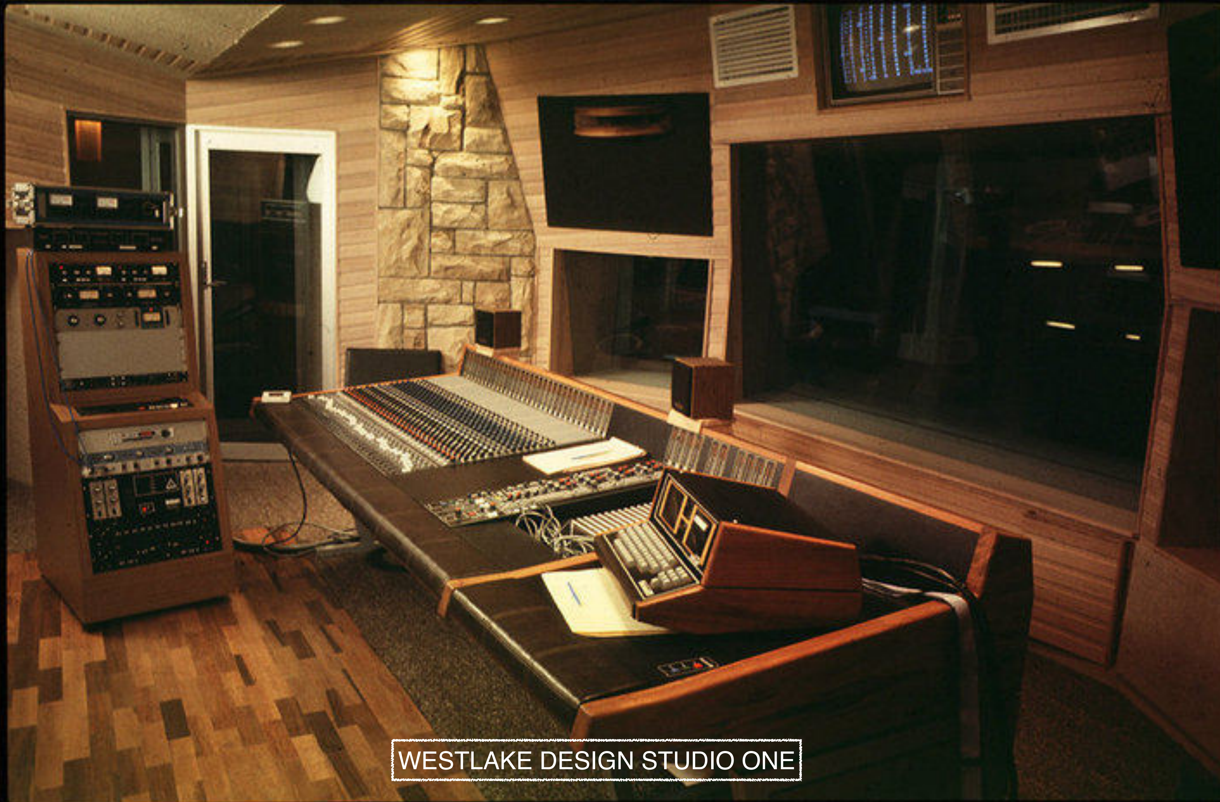
HARRISON 32 CHANNEL MR2 CONSOLE WITH COMPUTER VCA MIXING
